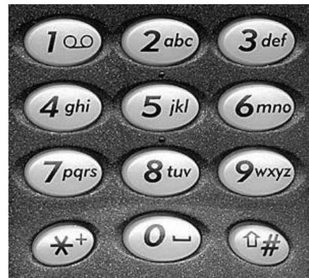
Figure 1. The standard 12-key telephone keypad
